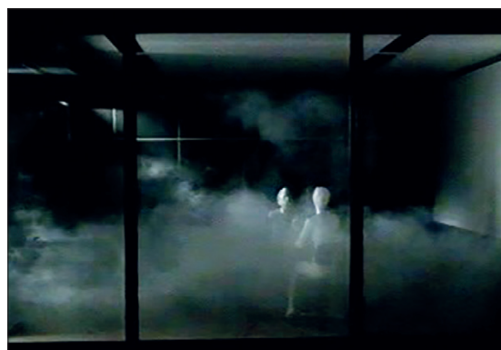
Air heated by occupants or equipment rises to high level
